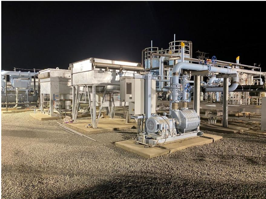
**Image 24.** Upgrader equipment at the CalBioGas West Visalia Cluster, which receives biogas from S&S Dairy.
